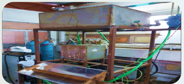
Standalone solar tea/coffee maker cum multipurpose water heating system
