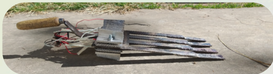
A low-cost Thermoelectric Generator based energy generating probe that can be used with existing stoves in rural villages in North-East India
